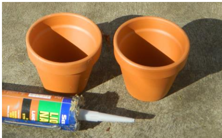
Step 1. Select two identical unglazed terracotta pots and seal one of the drain holes (for example, use silicone adhesive or masonry adhesive)
