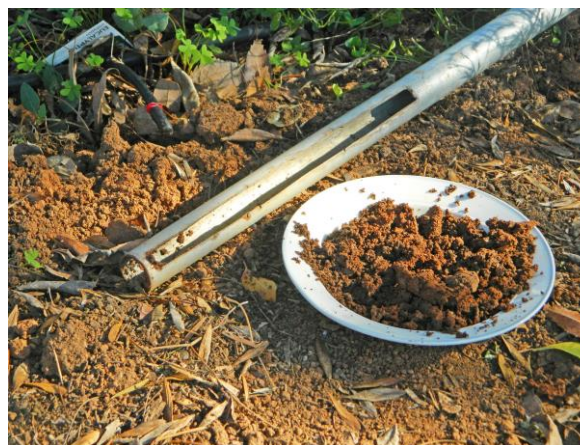
Measure the moisture content of the soil by weighing the moist soil, drying the soil in an oven, and then weighing the dry soil
