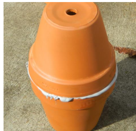
Step 4. Gently press the pots together and allow 24 hours for the sealant to cure
