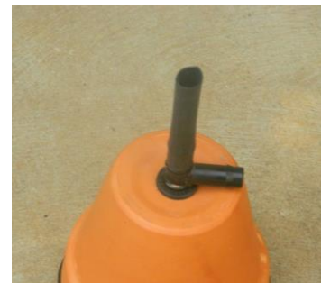
Step 4. Gently press the pots together and allow 24 hours for the sealant to cure
