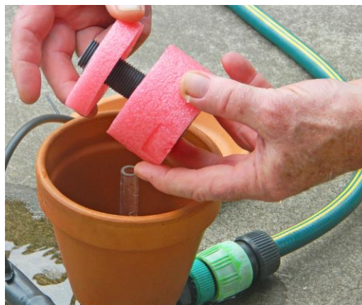
To adjust the interval between irrigation events, adjust the gap between the upper and lower float
