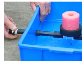
Attach the inlet adaptor to the inlet pipe
