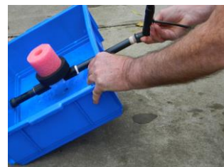
Attach the adjustable control dripper assembly to the outlet pipe
