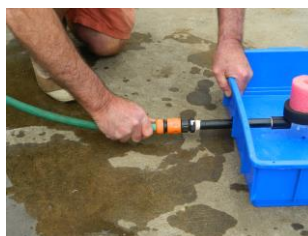
Connect the water supply to the inlet side of the evaporator
