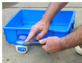
Lubricate one end of the pipe with Vaseline
