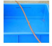
Step 3. Place a measuring container under one of the irrigation drippers.
