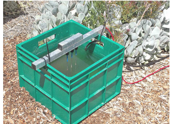
Evaporator and level sensor
