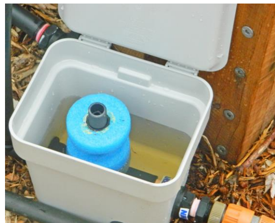
The water level in the controller is the same as the water level in the wicking bed.
