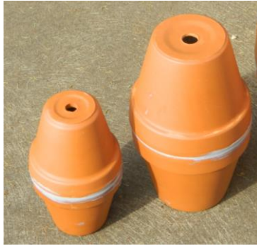
Small pitcher made from two 9cm terracotta pots (AU$1.27 each at Bunnings) Medium pitcher made from two 12cm terracotta pots (AU$1.76 each at Bunnings)
