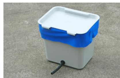
Adjust the interval between irrigation events by adjusting the exposed surface area of polyester cloth
