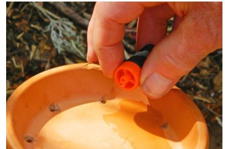
The control dripper is adjustable.
