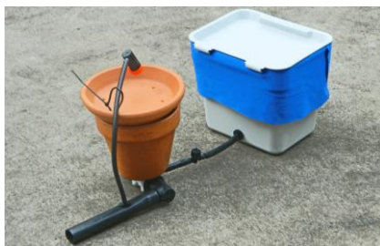
Booster connected to the drain valve on the terracotta pot
