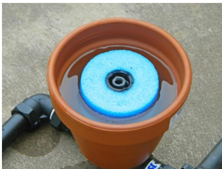
Float and the water level
