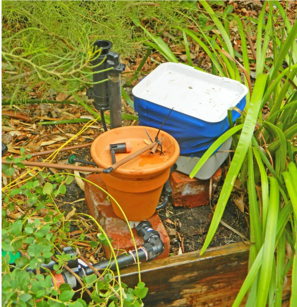
Terracotta Irrigation Controller for Solenoid Valves
