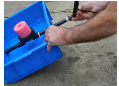
Connect the adjustable control dripper assembly
