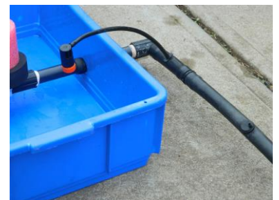
Connect the outlet to the irrigation application
