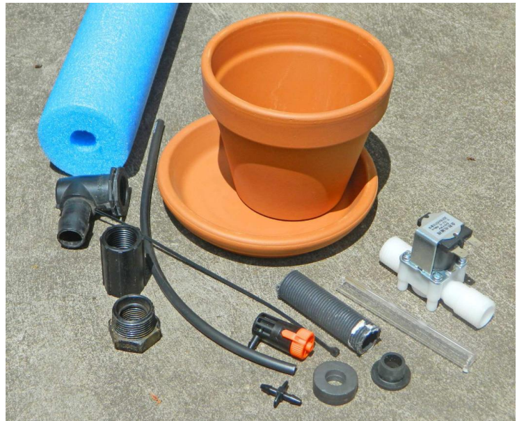
Components of the DIY Unpowered Irrigation Controller
