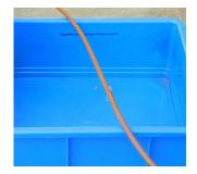
Step 3. Place a measuring container under one of the irrigation drippers.
