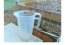
Step 4. The water level goes down as water evaporates from the evaporator. Use the irrigation system to replace the water that has evaporated. Stop the irrigation when the water level has returned to the level line. The amount of water in the measuring container is the amount of water discharged by each dripper during the irrigation event.
