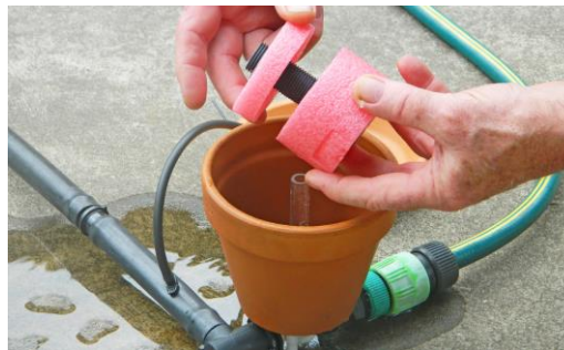
To adjust the interval between irrigation events, adjust the gap between the upper and lower float
